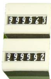
Figure 32 Mechanical Shot Counter
